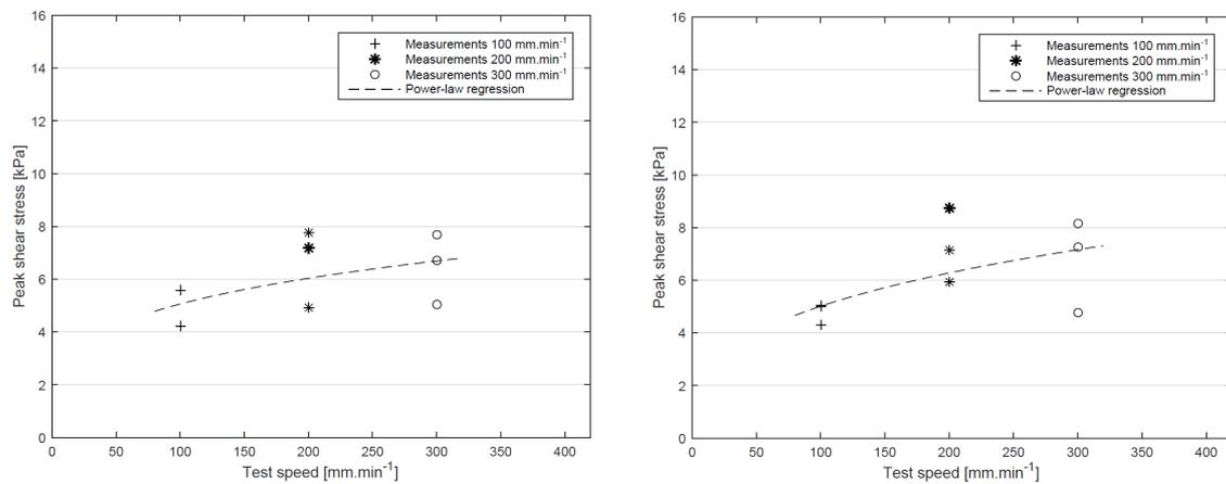
**Figure 3:** Evolution of peak shear stresses with respect to test speeds for inter-ply slip experiments (left)  $0^\circ/90^\circ$  (right)  $90^\circ/90^\circ$
