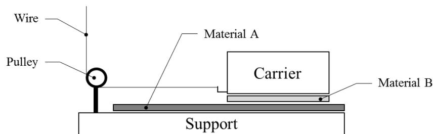
**Figure 1:** Schematic of the frictional test setup presented in DIN 14882 (adapted from [2])
